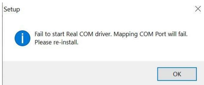
If there is a firewall between your Server and the NPort device (both Windows and Network firewall), please ensure that TCP Port 80, 950, 966 and UDP Port 4800 are open for your Moxa NPort device and assigned IP address.
