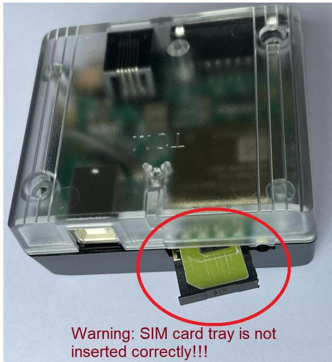
iv). To eject an inserted SIM card, simply slowly depress the yellow button so that the SIM card tray slides out.
